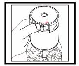
10. If the slow release valve is open and the sound of air coming out stops, press the fast release button to make sure pressure is fully released. (For water you can press the fast release button right any time)
